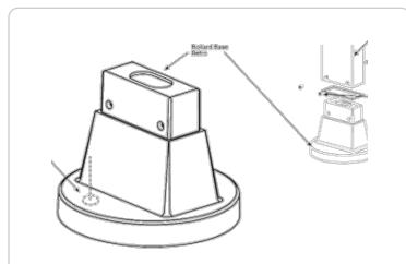
Bollard base adaptor for retro kit no mtg plate/bolts or bollard base adaptor  $\delta^{\prime\prime}$  round new w/ mtg plates and bolts.
